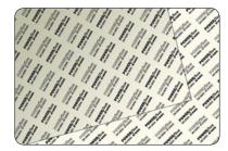
Structured PTFE - Gasket - Sheet manufactured by a unique process which provides a high level of fibrillation to overcome the creep relaxation and cold flow problem associated with normal (skived or moulded) PTFE sheets. POWER®flon 30 WHITE is produced from virgin PTFE resin filled with Barium Sulphate.
